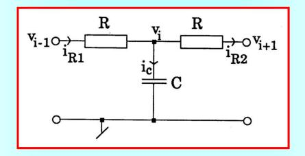
$$\frac{dv_{i}/dt = i_{C}/C}{i_{C} = i_{R1} - i_{R2}} \implies \frac{dv_{i}/dt = (i_{R1} - i_{R2})/C}{= (v_{i+1} - 2 \cdot v_{i} + v_{i-1})/(R \cdot C)} \implies \frac{(R \cdot C) \cdot \frac{dv_{i}}{dt} = v_{i+1} - 2 \cdot v_{i} + v_{i-1}}{\Rightarrow (R \cdot C) \cdot \frac{dv_{i}}{dt} = v_{i+1} - 2 \cdot v_{i} + v_{i-1}}$$
