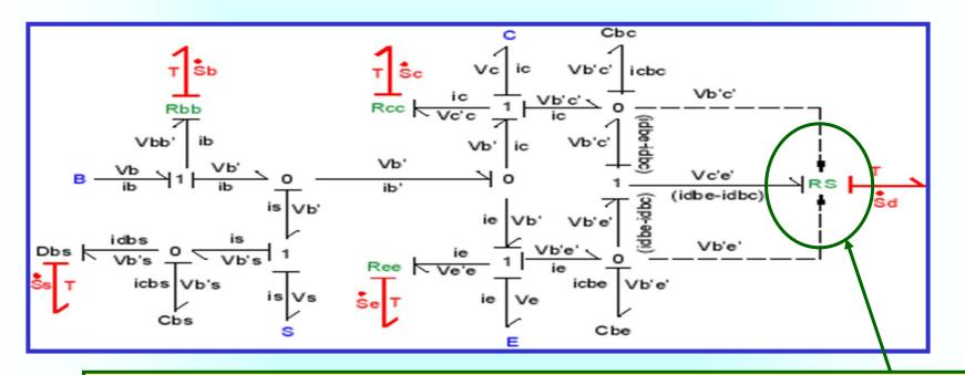
The two current sources are really a power sink, rather than a power source. They can be interpreted as a single non-linear resistor.
