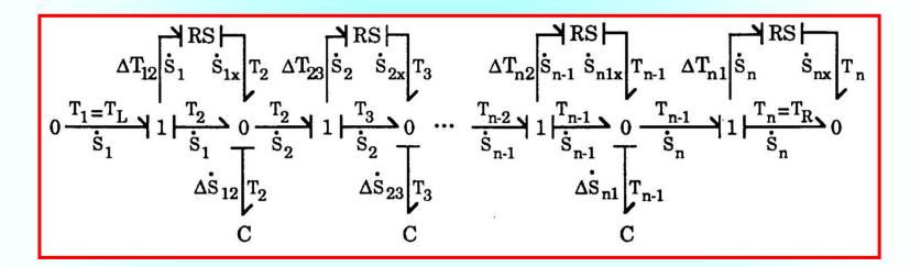
• The temperature gradient leads to additional entropy, which is re-introduced at the nearest 0-junction.
